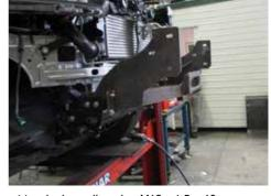
washers, spring washers and nuts. Fix cradle gusset to winch cradle using M12 x 1.5 x 40 bolts, flat washers, spring washers and M12 nuts. Centralize cradle to vehicle body.
